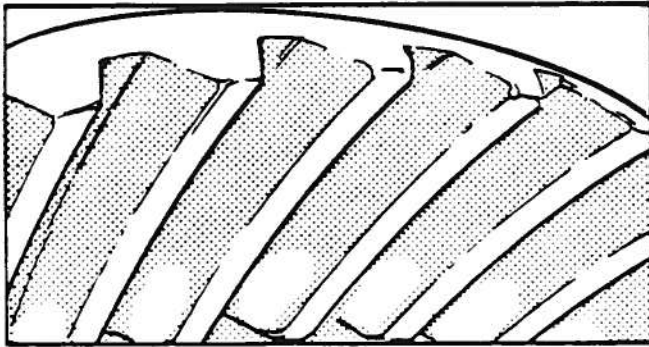
PATTERN "B" — CONCENTRATED BEARING AT TOE
