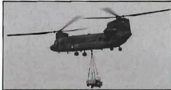
Figure 4. SATS during single point helicopter sling load testing with CH-47
