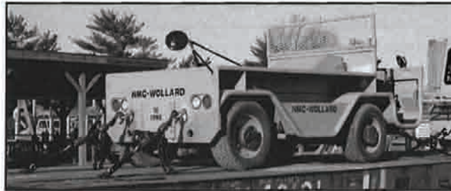
Figure 3. SATS secured to railcar (rear view)
