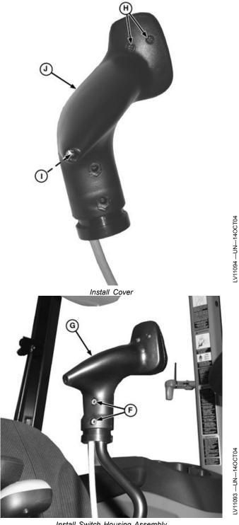
Install Switch Housing Assembly
