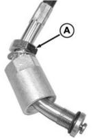
SCV Cable Retaining Nut
