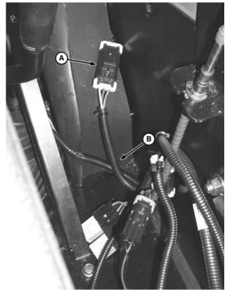
Connect Wiring Connector
