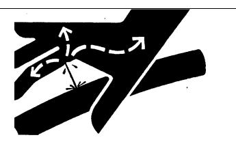
The hydraulic lines may leak when being disconnected. Contain leaking oil and dispose of properly.
