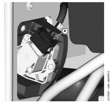
Foot Throttle Position Sensor—Cab
