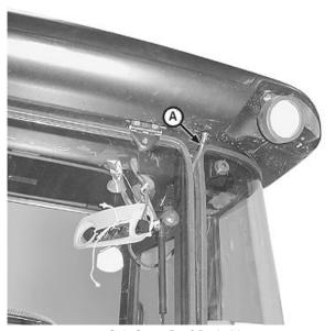
Cab Outer Roof Drain Lines
