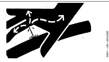
The hydraulic lines may leak when being disconnected. Catch leaking oil and dispose of properly.
