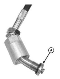
SCV Cable Retaining Nut
