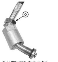
Rear SCV Cable Retaining Nut
