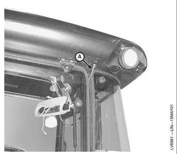
Cab Outer Roof Drain Line
