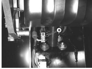
Clutch Disengage Switch Wiring Connector
