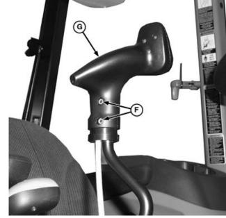
Remove Switch Housing Assembly
