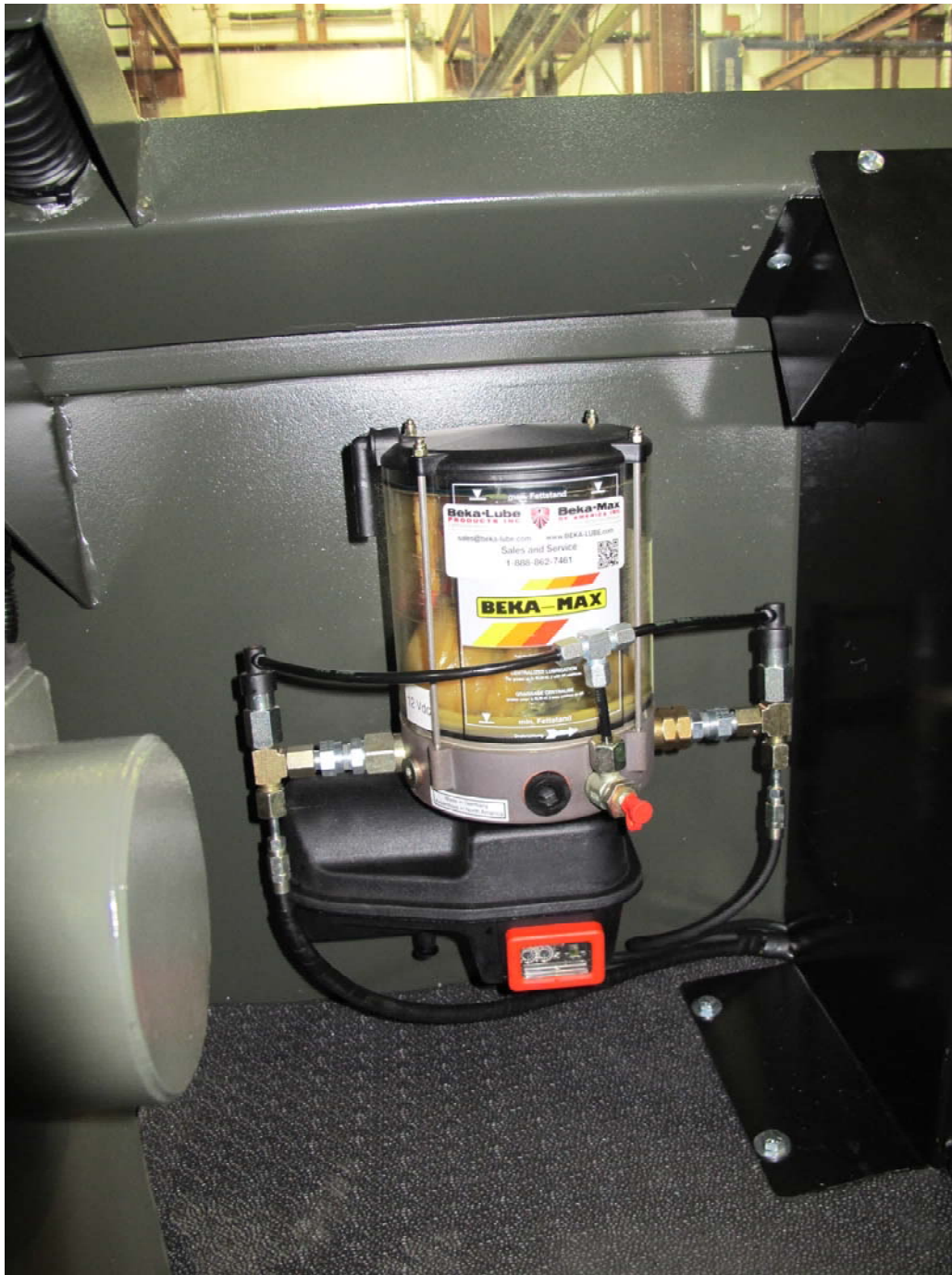
Pump mounted inside of the operator's cab.
