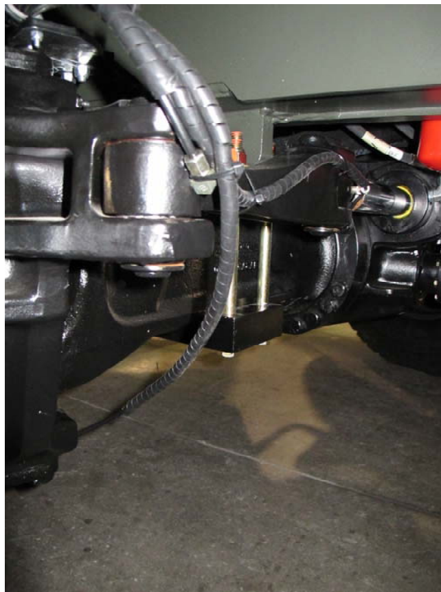
Note: Clamps mounted to plate and not to axle.
